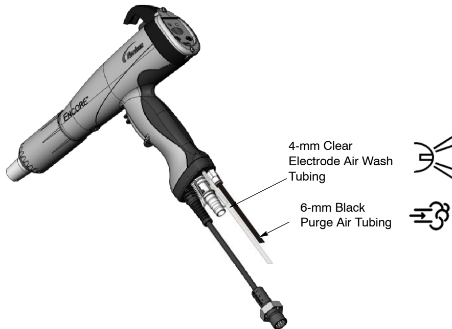
Figure 2-8 Connecting Purge and Air Wash Tubing to the Spray Gun
