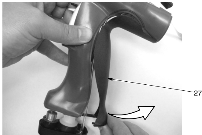
Figure 5-7 Removing the Ground Pad
