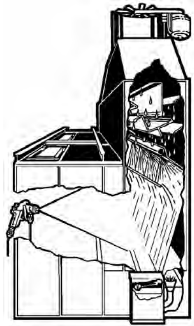
Figure 2 - Waterwash Type Spray Booth
