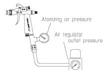
Pulling the trigger of the gun with the pattern adj. Set and fully opened adjust the air regulator in the spray booth to obtain 0.5~0.9 bar (7~13 PSI) at the gun inlet as issued on specifications table ahead. In this way the gun will atomize within 0.7 bar (10 PSI) inside air cap.
