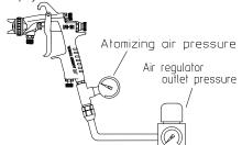
The gun should be held so that it is perpendicular to the surface of the work piece at all times. Then, the gun should move in a straight and horizontal line. Arcing the gun causes uneven painting.
