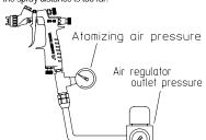
The gun should be held so that it is perpendicular to the surface of the work piece at all times. Then, the gun should move in a straight and horizontal line. Arcing the gun causes uneven painting.
