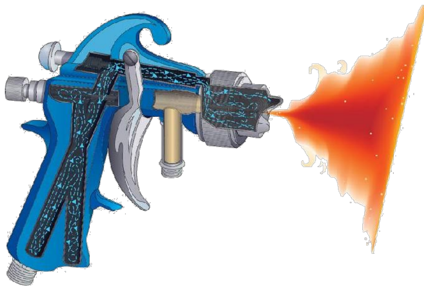
Figure 1: Sharp-cornered gun chambers in HVLP guns create turbulent air that reduces finish quality.
