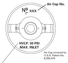
Maximum air pressure required to assure compliance of 10 PSI Max. Cap Pressure - this reading must be taken at the spray gun handle inlet fitting.
