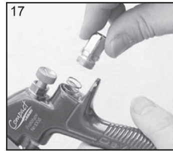
17. Replace Valve Spring and attach Housing (10).
