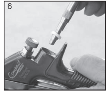
6. Remove Valve Seat.
