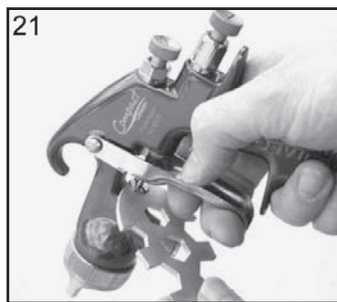
21. Adjust Needle Packing (4) with wrench sufficient to seal but to allow free movement of needle. Lubricate with gun oil.
