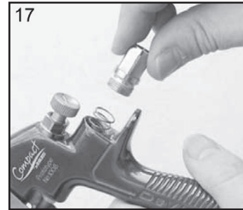
17. Replace Valve Spring and screw in Housing (10).
