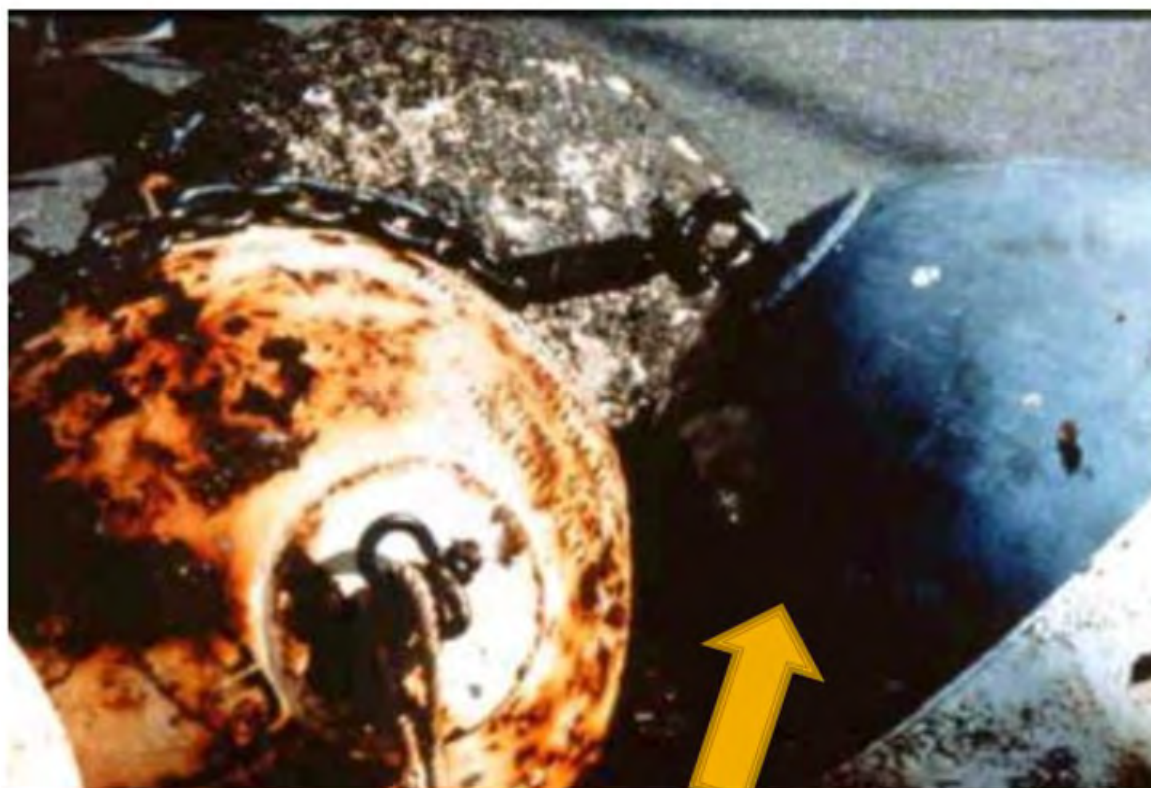
The bottom half of the buoy on the right was coated with NASA's zinc-silicate and shows no sign of marine growth after being submerged for two years.
