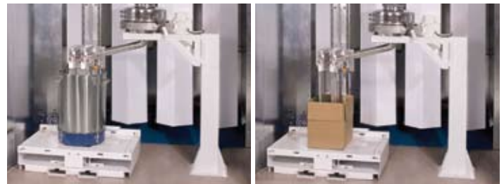
Capable of delivering powder from 50 lb. stainless steel round hoppers and powder supplier's boxes
