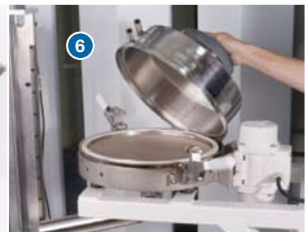
Capable of delivering powder from 50 lb. stainless steel round hoppers and powder supplier's boxes
