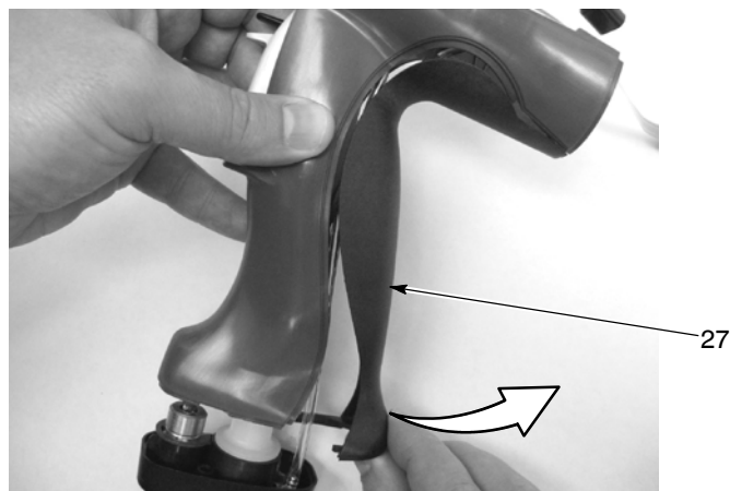
Figure 5-7 Removing the Ground Pad
