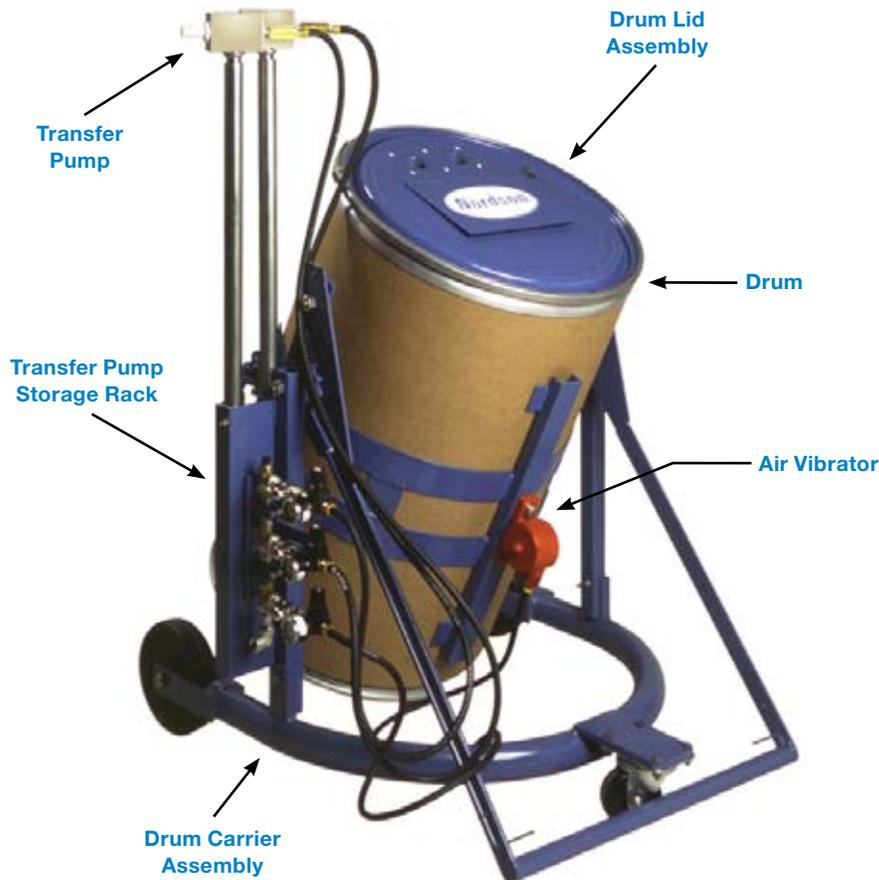
The patented Nordson bulk powder feed system supplies virgin powder directly from a fiber drum to a Nordson hopper/feeder. The system features a drum carrier unit, custom drum lid, and up to three powder transfer pumps, each capable of delivering up to 200 lbs. (91 kg.) of powder per hour.
