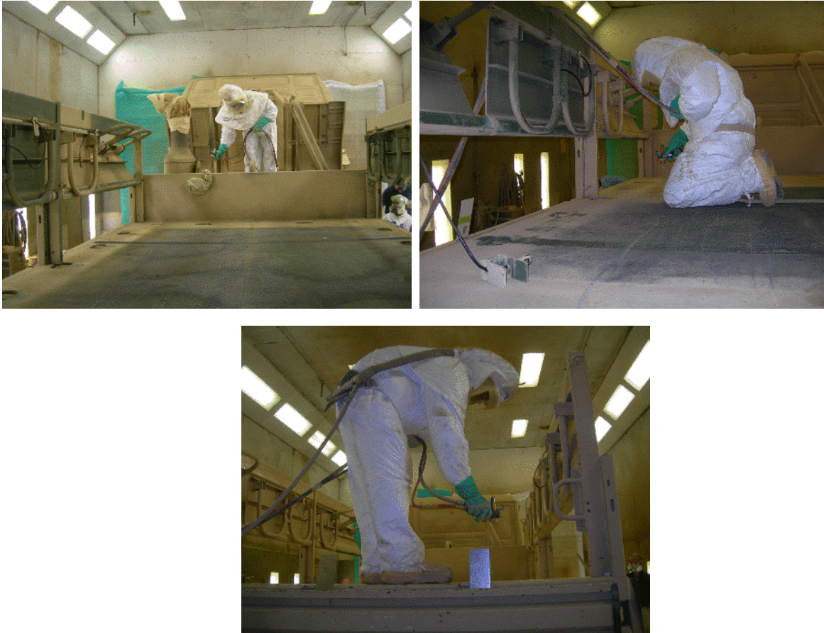
Figure 13. Painter applying coating using the DUX spray gun.
