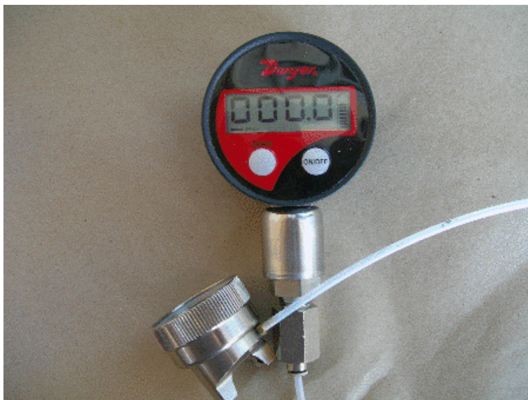
Figure 9. Close up of Dwyer pressure gauge and kit to measure atomizing pressure.
