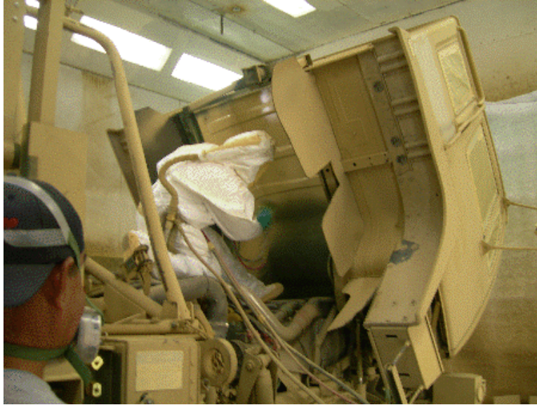
Figure 16. Painter applying coating to the underside of the LMTV M1083A1 vehicle hood.
