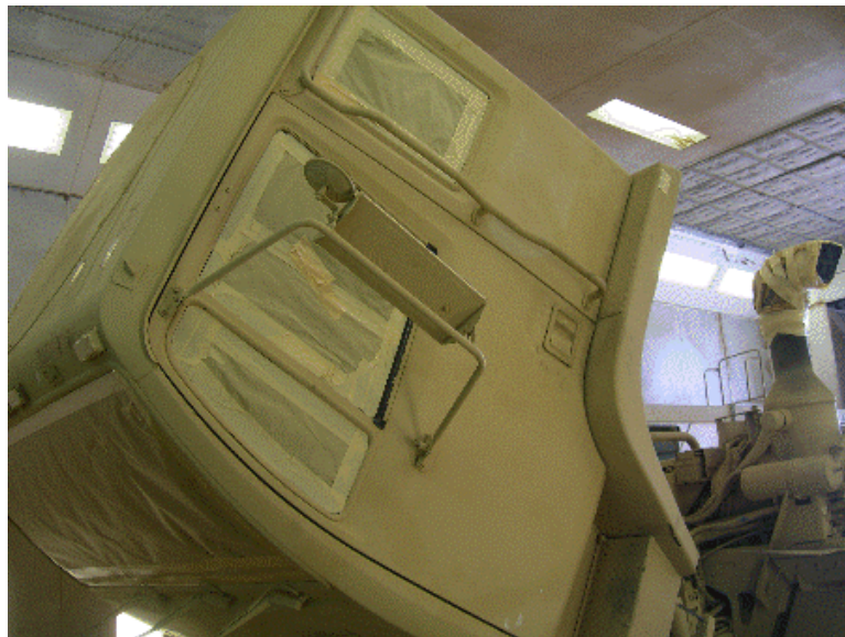
Figure 15. Hood of LMTV M1083A1 vehicle moved forward for painting.
