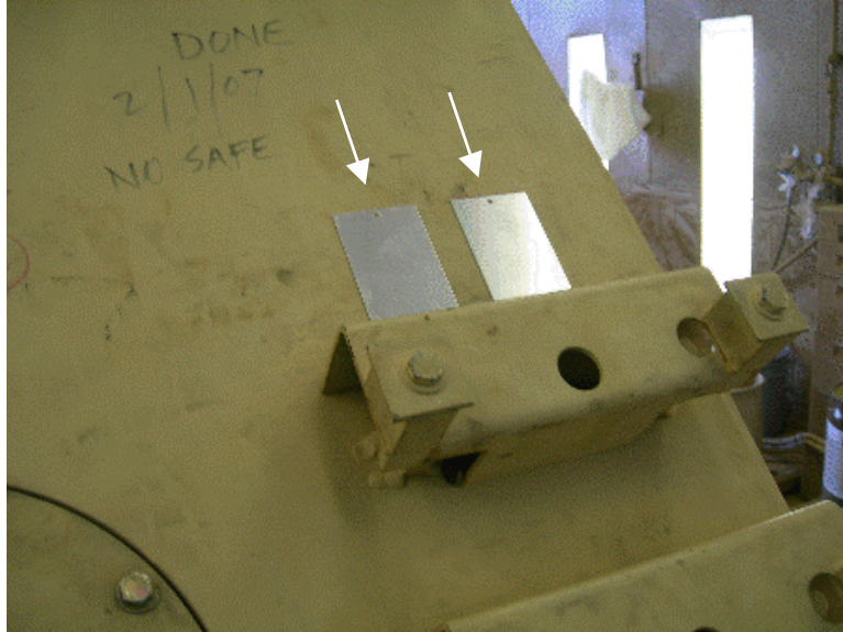
Figure 4. Small aluminum panels on the front of the M1068A3 vehicle used to measure dry film thickness.
