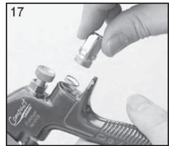
17. Replace Valve Spring and screw in Housing (10).
