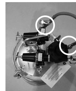
Assemble valve end of hose assembly to regulator using a 5/8 wrench. Assemble other end of hose to air motor with same wrench.
